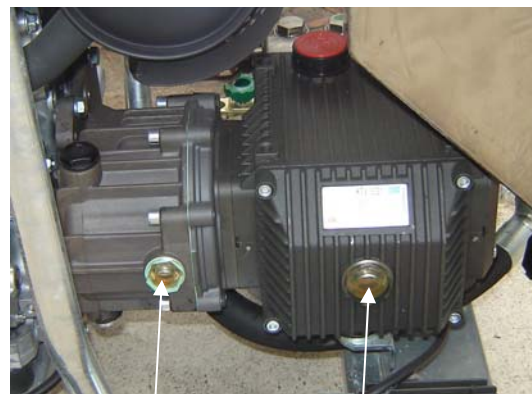
Gearbox sight glass
